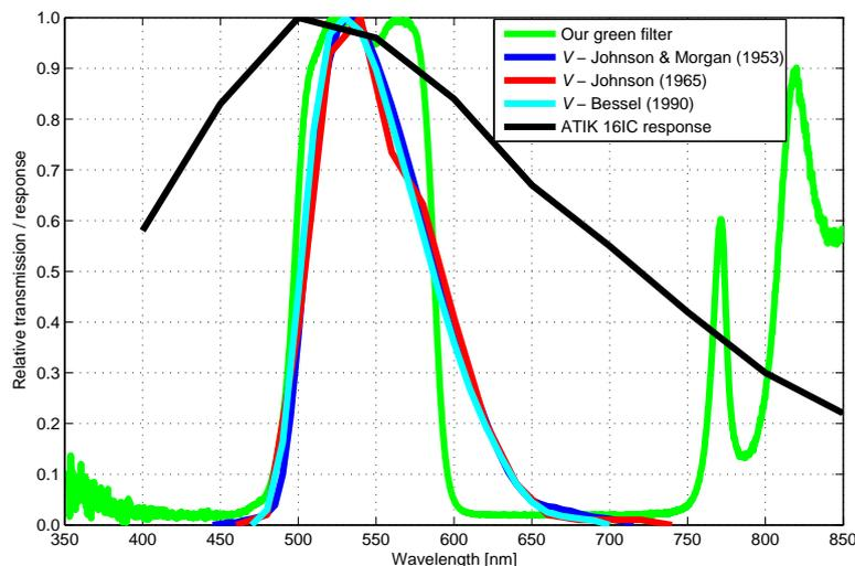
**Figure 1.** Relative transmission in the range of 350–850 nm for our *green* filter (own measurement) and for the standard photometric filters from the Asiago database together with the relative spectral response of the used ATIK 161C CCD camera.
